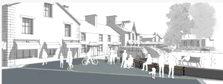
Visualisations of Section 3 Within Grasmere, with pedestrians, cyclists and vehicles sharing the space around the Easedale Road junction. A section of footway is created with new seating and cycle parking.
