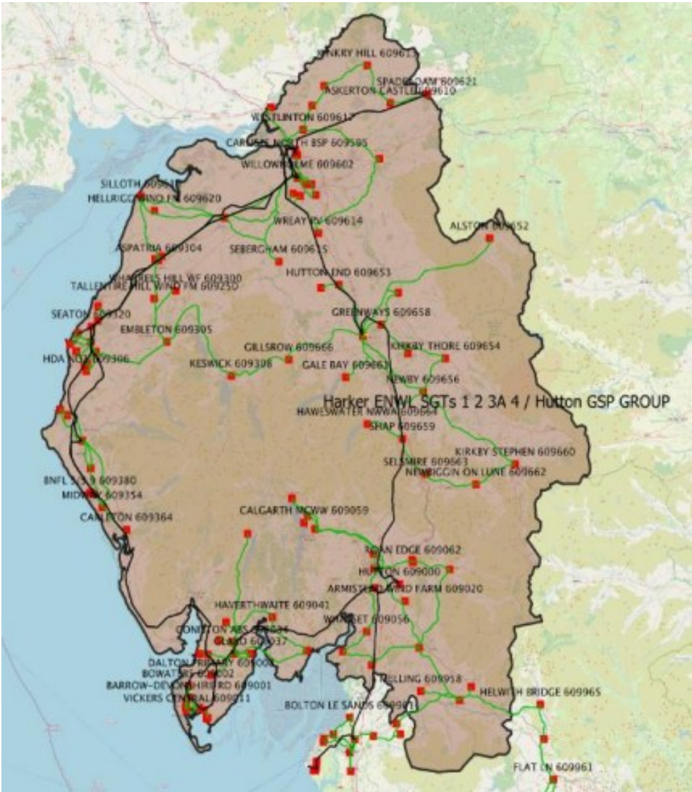
Figure 6.3: Electricity network serving Cumbria
